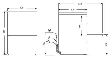
Power supply 240 V Total power 3.2 kW Total current 15 amp Wash tank capacity 20 ltr Rinse water consumption (per cycle) 1.5 ltr Rinsing temp (approx) 80-85 °C Rack size 500 x 500 mm Tallest washable glass 36.5 cm Weight (empty) 55 kg Water connection 3/4" hose
